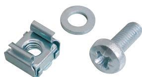
Cage nut M6, screw M6x16, washer 6.4
