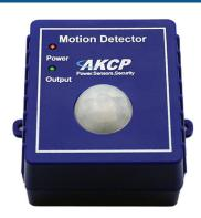
Infrared motion detection, is a hardware based motion detection technology that will detect movement up to 3 meters away. MD00 can be daisychained together with a maximum of 10 in a single string, meaning a single sensor port can support 10 motion sensors. When one motion sensor in the string is in critical state the whole string will show as critical.
