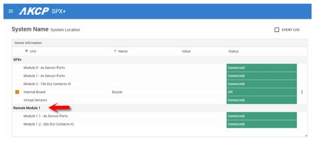
After connecting the BEB unit, this now appears as the "Remote Module" as you can see in the screen shot above. Now the sensors and notifications and dry contacts can be configured normally.
