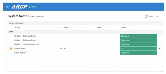
The screen shot above shows the SPX+ web UI before the BEB unit(s) are connected.
