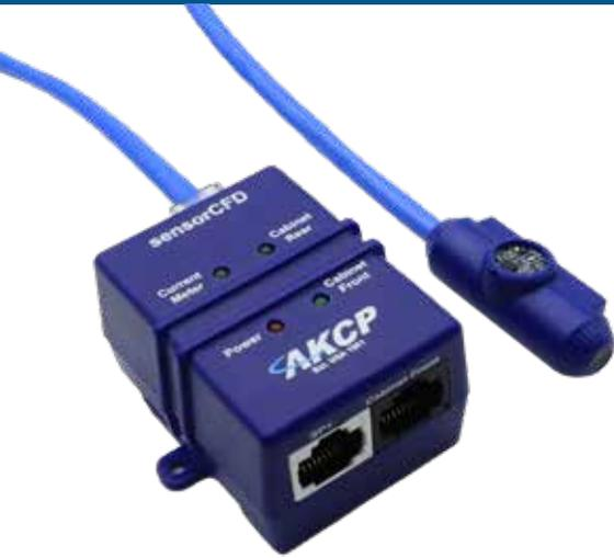
Pre-wired for easy installation on your cabinet. Placed at the top, middle and bottom - front and rear of the cabinet. This configuration of sensors gives monitoring of the air intake and exhaust temperatures of your cabinet, and the temperature differential from the front to the rear.
