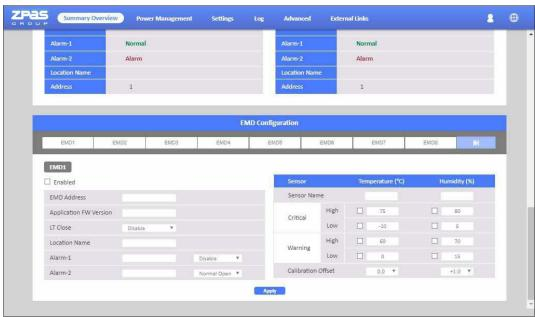
ZPAS GROUP PDU supports 8 EMD sensors in cascade each one with 2 digital inputs of . you can set 2 alarms for each EMD sensor. There are 3 op ons(Normal Open/Normal Close/Disable) of the EMD sensor. If you set "Normal Open", the EMD sensor will become "Warning"(Yellow light) when closed.
