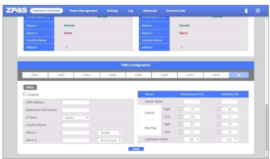
ZPAS PDU supports 8 EMD sensors in cascade each one with 2 digital inputs to set 2 alarms for each EMD 31 sensor. There are 3 options(Normal Open/Normal Close/Disable) of the EMD sensor. If you set "Normal Open", the EMD sensor will become "Warning" (Yellow light) when closed.
