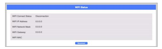
**Step 4:** Please access the dongle IP address and make sure the Wi-Fi or 3G/4G dongle is workable.
