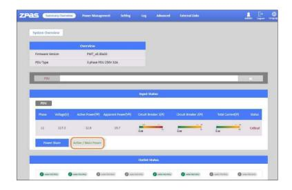
**Step 3:** When PDU A has utility power fail, the status of power share will display **Active/Backup Power** on the **System Overview** webpage.
