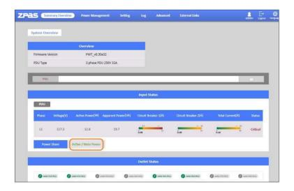
**Step 4:** At the same, the information of inlet phase load management will not display on the Inlet **Configuration** of the **Power Management** webpage.
