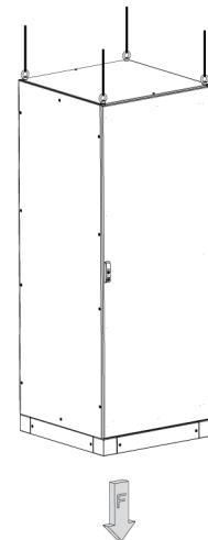
9 000 N if cabinet lifted by 4 lifting eyebolts
